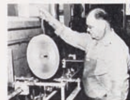
A newly recorded acetate disc is given a thin coating of silver and immersed in a plating tank to make a metal master. A metal mother, and later a stamper will be made.
