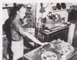
The sound from the studio is carried to magnetic tape recorders which reproduce sound impressions on tape.
