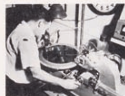
Music from the tapes are re-recorded on acetate discs. Fine microgrooves are cut in the lacquer master, and studiously inspected by microscope.
