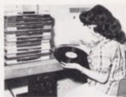
Careful visual inspection of each record for molding defects in the manufacturing process is a prime requisite.
